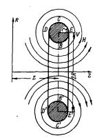
We shall first consider the question qualitatively. We shall suppose that a vortex ring with a current (figure) has formed in the gas, and that the magnetic lines of force and the stream lines for the vortex flow are directed as shown in the figure. The current flowing in the ring excites a magnetic field in the ring which is determined by the Biot-Savart law
